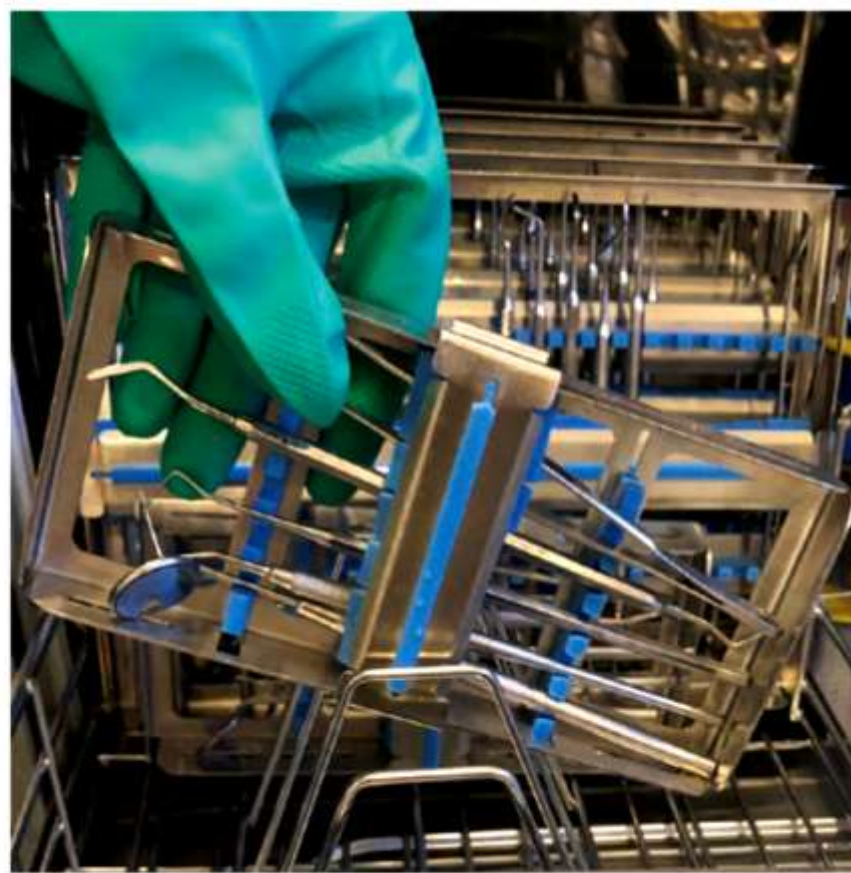
Fig. 6.5 Instrument cassettes loaded in a thermal washer disinfecter
